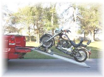
♦ The effort free, unique return system pulls the motorcycle back out of the bed. No need for a second or third winch with confusing electronic switching. The system incorporates a hand held remote switch with 15 feet of cable.
